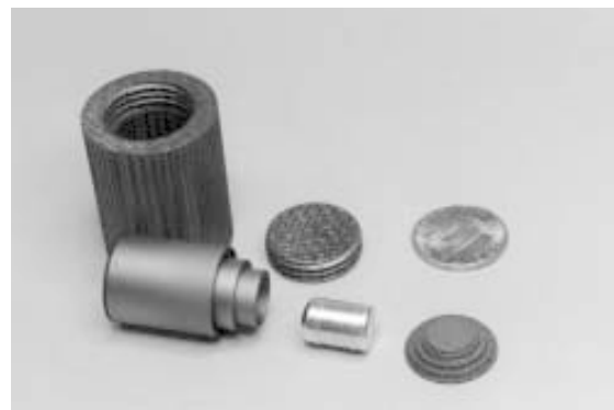
A Light Weight Radioisotope Heater Unit (LWRHU) before final assembly. The heat source consists of a graphite aeroshell, pyrolytic graphite thermal insulators, and a platinum-rhodium fueled clad. A sintered platinum powder frit vent is electron-beam-welded into the end cap of the fueled clad to release helium generated by the alpha decay of the fuel.
