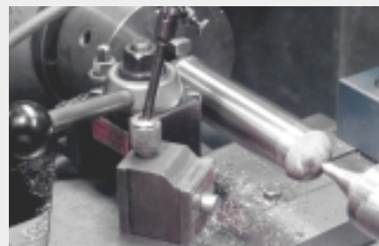
A plutonium rod is being machined on a lathe.
