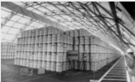
Transuranic waste in interim storage at the Idaho National Environmental Engineering Laboratory. These barrels are to be shipped to WIPP.
