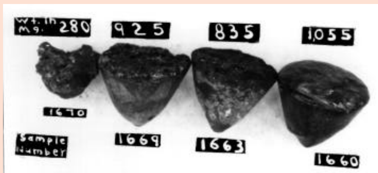
Figure 2. Four more plutonium metal buttons made by Magel and Dallas during the spring of 1944.
